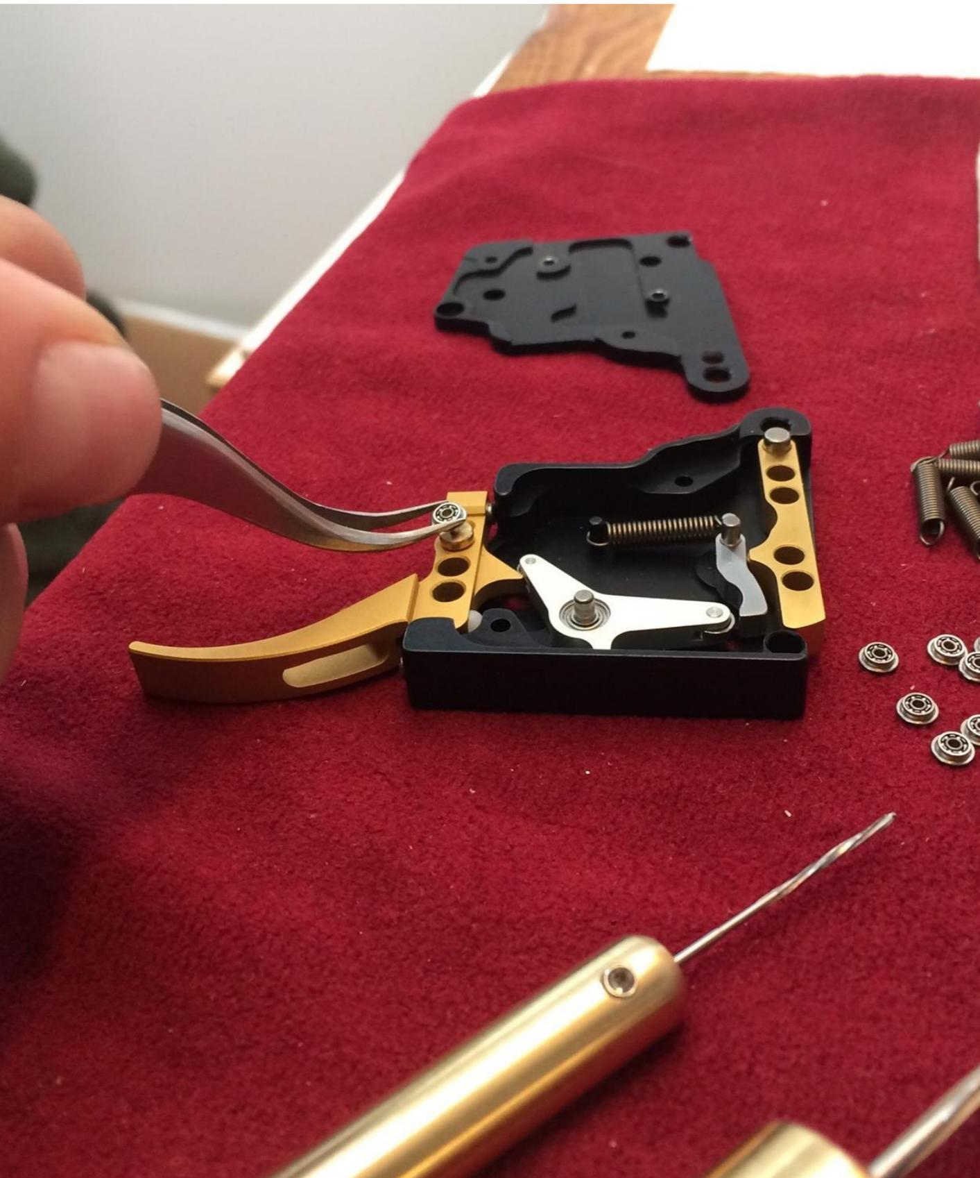
Assembly of the triggers is handmade by experienced staff.
