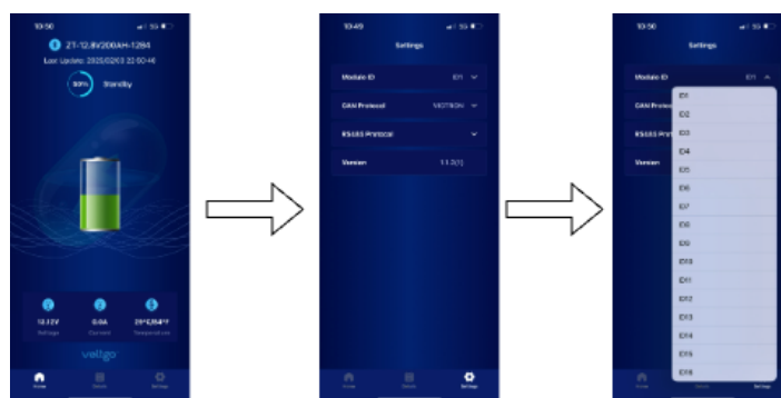
Figure 11. VoltGo battery app to change battery ID number.
