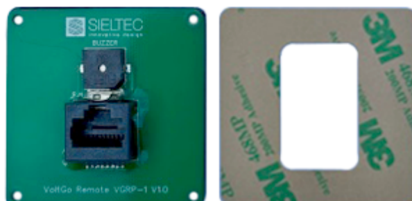
Figure 4. Remote panel mounting adhesive
