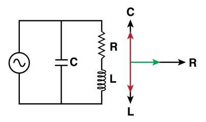
In this case we have corrected a power factor problem by introducing a reactive load of opposite phase into the circuit, in parallel with the original load. Notice the inductive reactance and the capacitive reactance are equal and opposite, cancelling and only leaving the in-phase resistive component.
