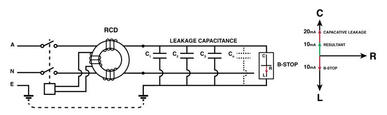
The choice of inductive current level is important because too little does not nullify the capacitive current sufficiently. Too much (say over 20mA) and the RCD will trip because of inductive current if all other loads are disconnected. In that case the RCD would trip if all breakers on the switchboard were opened. What is required is a midpoint where the trip margin is restored without causing a problem because of the introduced inductive current vector.
