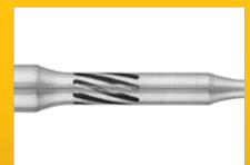
Helical reliefs redirect the ultrasonic energy from purely longitudinal to combined torsional component so tissue distal to the tip is unaffected by cavitation.
