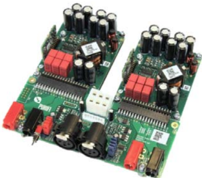
Purifi "EVAL1 is a kit combining two 1ET400A amplifier modules and a stereo front-end board
