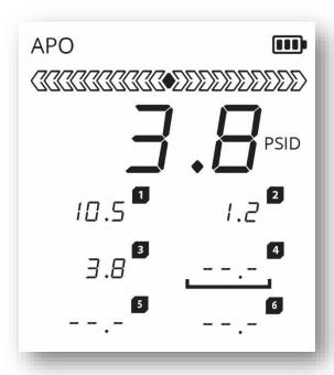
The active capture slot (where the next reading will be captured) is shown by an active position cursor. Position 4 in the example display above.
