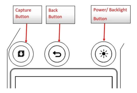
Capturing values allows you to eliminate the need for a pencil and paper at each assembly. Six values can be captured in memory and on the display allowing you to capture the working pressure as well as all test values on any backflow assembly. The capture button allows the tester to focus on the backflow assembly rather than the gauge, crucial for recording the relief valve or air inlet valve opening points.
