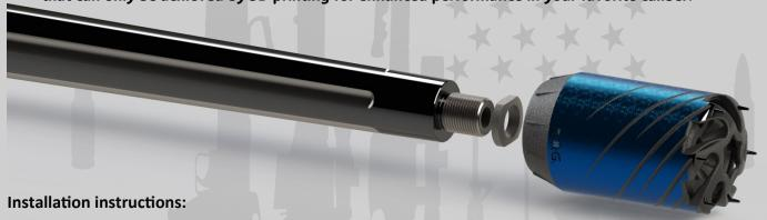
Prior to installation be sure the barrel threads are completely clean and undamaged. Screw included thread timing nut onto end of barrel until it stops at shoulder. Then thread the compensator onto barrel until it stops. Rotate the DEADSTOP back until the arrow is at the top. Using a wrench back the jam nut up to meet the compensator with approx 15 ft lbs and secure its proper alignment position.
