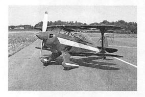
S/N 1021 - 1520 TTAF, 130 hours Since Aviat Factory Rebuild. New lower wings, new gear, new tires, brakes, new stearable tailwheel, new fuel tank, many others.
