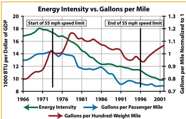
This comparison reveals important distinctions in the evolution of passenger and freight efficiency. The graphs, representing gallons per passenger mile and gallons per hundred-weight mile, are normalized to 1 for the year 1974, when the federal 55 mph speed limit was imposed.
