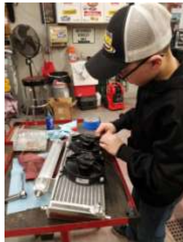
Noah installing the SPAL fans on the new oil cooler going on his asphalt car. We are always looking to upgrade our cars to make them the most competitive on the track!
