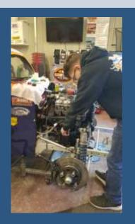
Noah installing the motor mount on the rebuilt motor.
