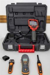
The Mold Busters process introduces new mold inspection tools (clockwise from top): borescope (camera/viewing device for tight spaces), hygrometer (humidity detector), prolometer (surface moisture detector) and anemometer (airflow detector).
