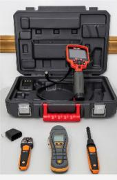
The Mold Busters process introduces new mold inspection tools (clockwise from top): borescope (camera/viewing device for tight spaces), hygrometer (humidity detector), proliometer (surface moisture detector) and anemometer (airflow detector).
