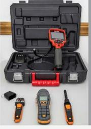
The Mold Busters process introduces new mold inspection tools (clockwise from top): borescope (camera/viewing device for tight spaces), hygrometer (humidity detector), prolometer (surface moisture detector) and anemometer (airflow detector).
