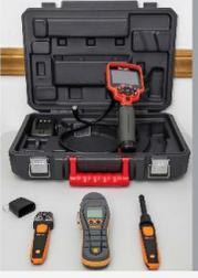
The Mold Busters process introduces new mold inspection tools (clockwise from top): boroscope (camera/viewing device for tight spaces), hygrometer (humidity detector), prolometer (surface moisture detector) and anemometer (airflow detector).
