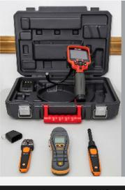
The Mold Busters process introduces new mold inspection tools (clockwise from top): borescope (camera/viewing device for tight spaces), hygrometer (humidity detector), protimeter (surface moisture detector) and anemometer (airflow detector).
