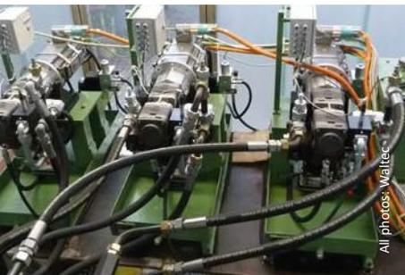
Unlike conventional valve hydraulics, the servo pump directly transmits the energy from the drive motor to the hydraulic press cylinder. In other words, the servomotors provide only the energy that is needed for each phase of the press process.
