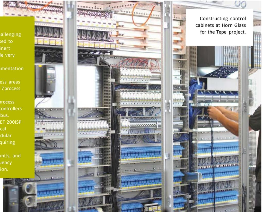
Constructing control cabinets at Horn Glass for the Tepe project.
