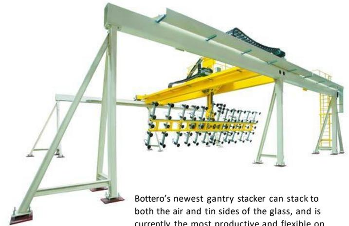
Bottero's newest gantry stacker can stack to both the air and tin sides of the glass, and is currently the most productive and flexible on the global market.
