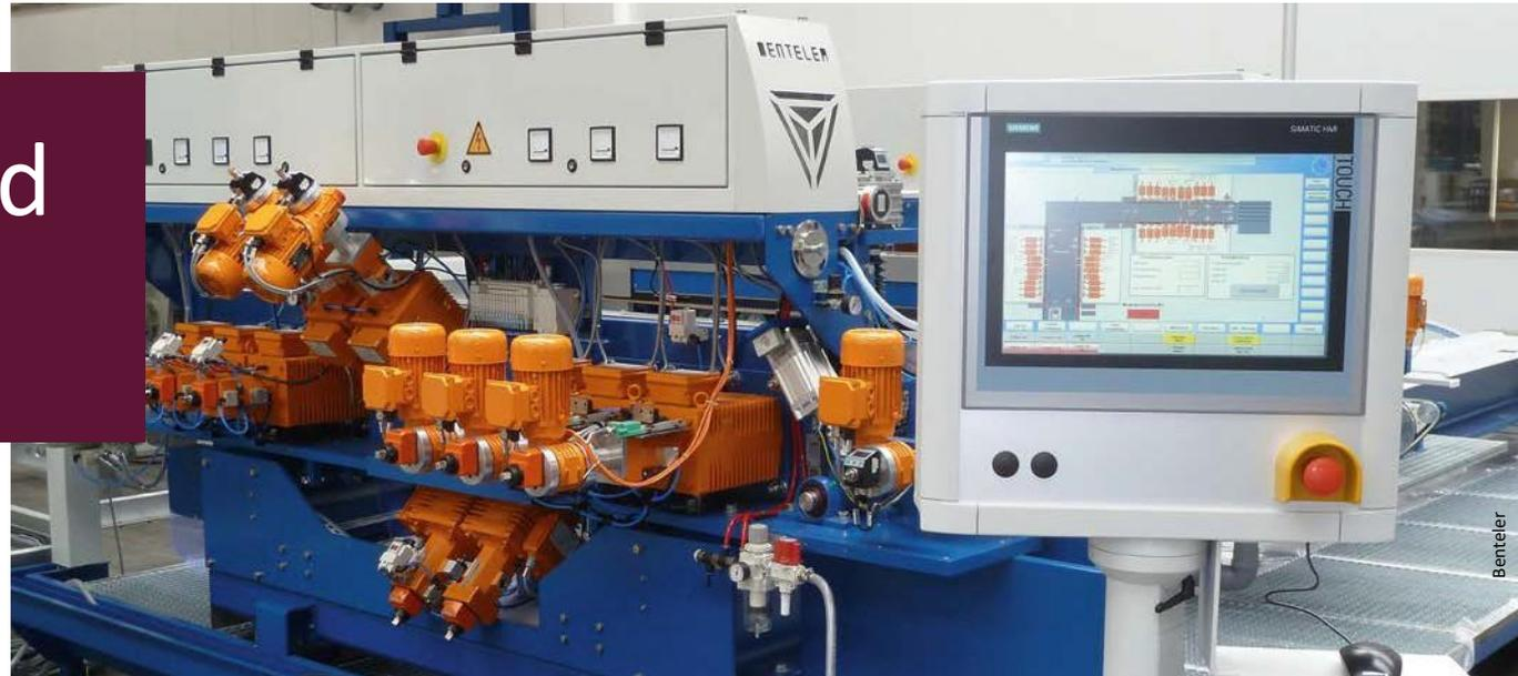
Industry insiders know that the globally operating Benteler Group has a German subsidiary in Bielefeld that specializes in the manufacture of glass processing machines, among other products. For example, Benteler Maschinenbau GmbH produces fully automatic, modular production lines for loading, cutting, breaking, grinding, and drilling both flat and curved glass of practically any type. The company has long relied on control and drive technology from Siemens.
