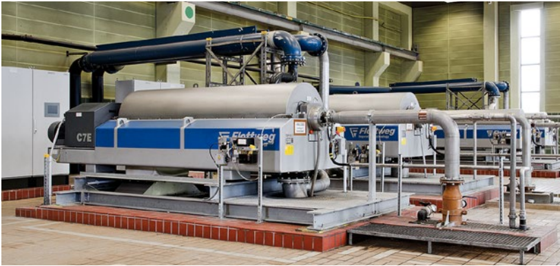
The decanter centrifuges at Flottweg in Vilsbiburg have been equipped with the Simatic S7-1200 fail-safe Basic Controller since the end of 2016
