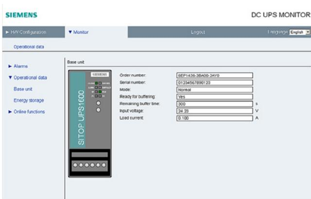
The password-protected web server supports viewing of the configuring and operating data.
