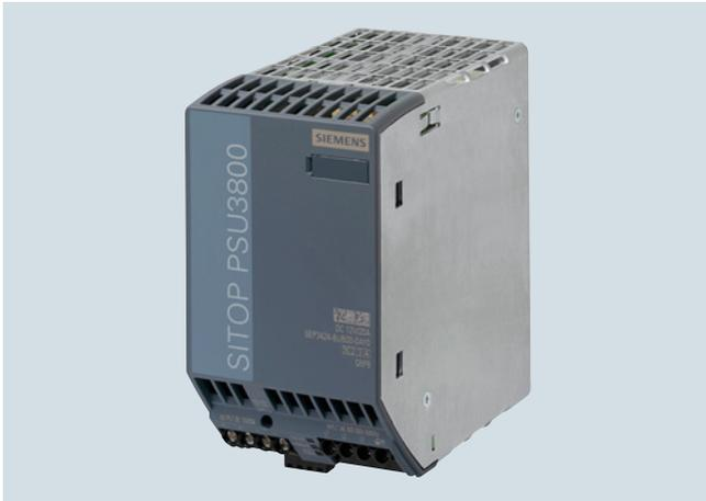
The SITOP PSU3800 3-phase power supplies are suitable for battery charging, thanks to their constant-current characteristic. For other applications, the output characteristic can also be switched to latching shutdown. The three-phase, wide-range input enables them to be used worldwide. The slim design requires little space on the DIN rail. Installation gaps are not required.
