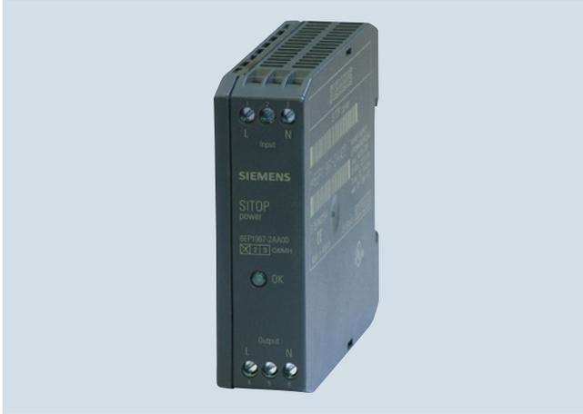
The SITOP inrush current limiter is used to reliably reduce the starting currents that are caused, for example, by transformers or with pulse-controlled power supplies by the rectifier circuit on the input side with capacitor charging.
