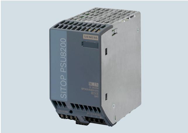
The 3-phase SITOP modular are technology power supplies for sophisticated solutions and offer maximum functionality for use in complex plants and machines. The wide-range input allows a connection to almost any electrical power system worldwide and ensures a high degree of safety even if there are large voltage fluctuations. The power boost provides up to three times the rated current for brief periods. In case of overload, you can choose between constant current with automatic restart or
