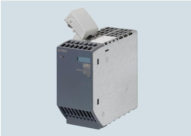
The BUF8600 buffer modules with maintenance free energy storage units are part of the SITOP PSU8600 modular system and are designed to bridge short-term power failures. They automatically take over the DC power supply in case of a line voltage failure. You can connect up to two BUF8600 buffer modules to the PSU8600 basic unit. Connection takes place on top of the modules without any wiring by means of the System Clip Link, a connecting plug for system data and power supply.
