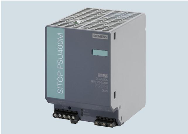
The SITOP PSU400M power supply with a 600 V DC input is suitable as an efficient DC/DC converter for drive and battery systems; large input range and temperature range, high efficiency; slim design; with 50% extra power for 5 s/min.
