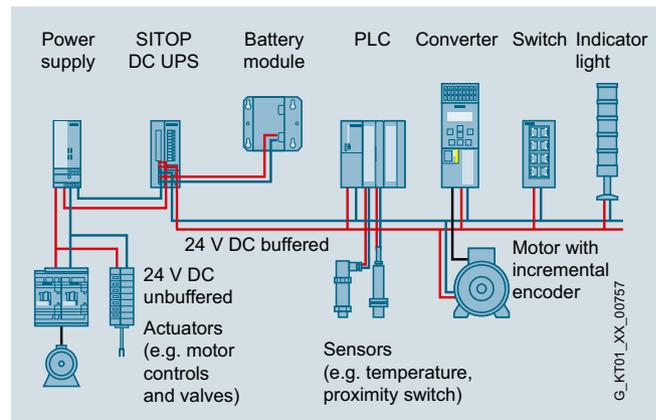
Configuration with SITOP DC UPS and battery module: 24 V buffering to maintain communication, signaling and sensor measured values. To relieve the load on the UPS, the actuators are supplied directly from the power supply unit.
