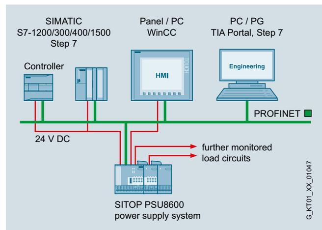
An extremely high level of reliability is achieved for the DC voltage supply by monitoring the individual DC branches for overload and bridging short-term power failures (brownouts). Complete transparency and fast fault localization are achieved by providing comprehensive diagnostic and maintenance information (e.g. load states of the outputs, phase/network failure, overtemperature) via PROFenergy.
