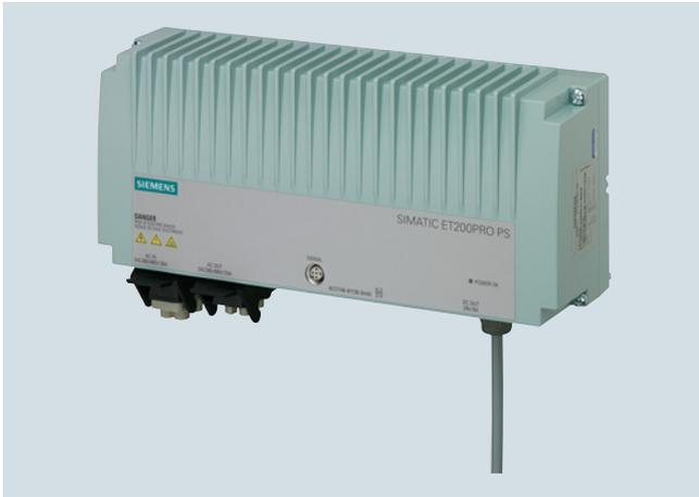
The SIMATIC ET200pro PS power supply unit with degree of protection IP67 is used as the electronics/encoder supply and load voltage supply of the new SIMATIC ET 200pro distributed I/O system for use close to the machine without a cabinet. With a signaling contact for "24 V OK" and "Overtemperature", as well as a second plug-in connector for input voltage loop-through.
