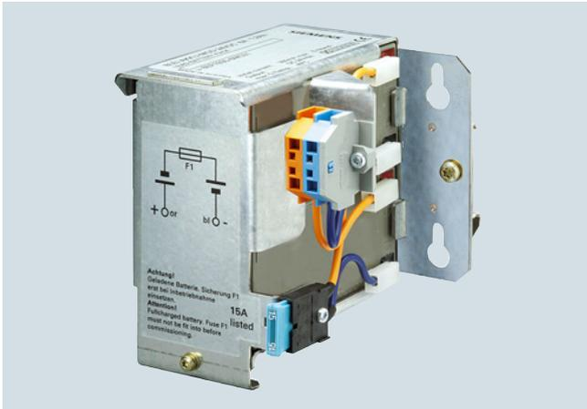
Maintenance-free battery modules with 1.2 Ah up to 12 Ah (lead-gel accumulator) for ambient temperatures from 0 to +40 °C as well as high-temperature battery module with 2.5 Ah (pure-lead accumulator) for ambient temperatures of -40 °C to +60 °C. The battery modules are completely prewired with battery retainer and terminals. For longer buffer times, the battery modules can be connected in parallel. Mounting onto standard mounting rail or directly to the wall.
