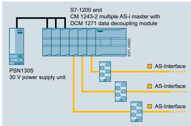
Configuration of AS-Interface multiple networks, each with one PSN130S 30 V power supply unit (examples with schematic representation):
