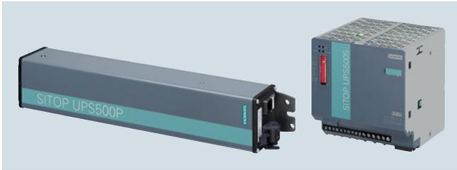
SITOP 24V power supplies can be expanded with a SITOP UPS500 uninterruptible DC power supply (DC UPS) for bridging short-term power failures in the order of minutes. For PC-based automation solutions, the high-capacity double-layer capacitors of the SITOP UPS500 supply enough energy to back up the operation and application data and to shut down software applications in a defined manner. You can increase the buffer times using SITOP PSU501S expansion modules (up to 3).
