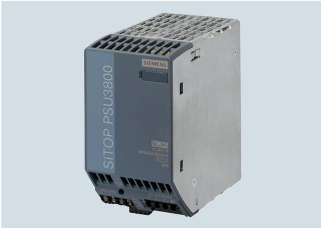
SITOP PSU3800 3-phase power supplies (24 V DC/17 A and 30 A) are suitable for battery charging, thanks to their constant-current characteristic. For other applications the output characteristic can also be switched to latching shutdown. The three-phase, wide-range input enables them to be used worldwide. The slim design requires little space on the DIN rail. Installation gaps are not required.
