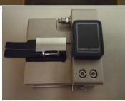
**B** Place the prepared fibers into the holding trays as shown here: Lower the Y wedge and hood.
