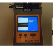
A Power on by touching the power/splice button, touch menu>calibrate>select OK *Auto calibrates* for all environmental factors and
