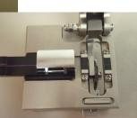
your fiber quality. Hinge the hood, and the Y wedge up, remove the sample fiber and prepare it and another fiber by stripping, cleaning (with prep wipe) and cleaving the ends by rapidly "flicking" the blade back from a forward rest position with the cleaver cover closed.
