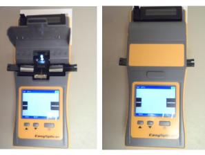
C Place protected splice in Oven (lift cover with left lever) Hit Oven, the 60 sec heating cycle
