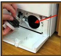
Washer Pump Clean-out
