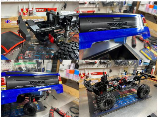
Ensure all bolts that were removed are tight, all link ends are tight, and your suspension clears correctly. Your truck should now be able to clear 2.2s. Minor trimming can be done to the fenders, rock sliders, and side trays to clear larger tires if needed.
