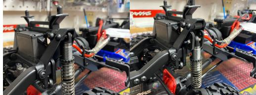
Next replace the servo bracket. You must remove the front bumper, shock towers, factory servo bracket, servo, and top of the receiver box to do so. The servo will now mount on the bottom of the bracket instead of the top so the wire needs to be unplugged from the receiver box prior to installation. This is a good time to upgrade the servo or at a minimum install a metal horn if you are planning on running larger tires.
