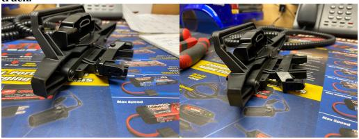
O the same on the rear bumper. Remove the bumper, flip the mount, and reinstall the mount. You will also need to slightly trim the rear of the body to accommodate the bumper mount being higher. Adjust both the front and the rear body mounts to raise the body. The mounts should be mounted in the second screw hole from the bottom.
