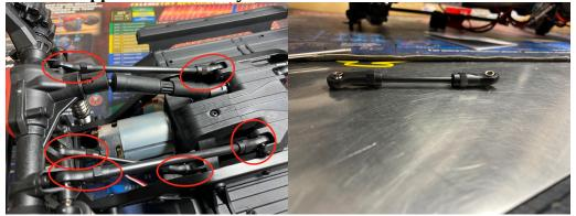
Remove front driveshaft and replace with longer included shaft. Ensure the marks on the driveshaft are lined up prior to reinstallation.
