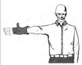
BOOM UP AND LOWER THE LOAD
