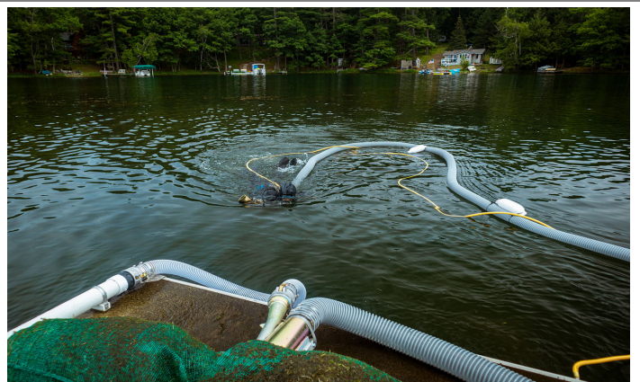
Photograph 3.3-4. Manual Removal with DASH. Photo credit Aquatic Plant Management, LLC.
