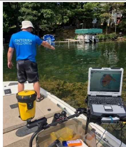
Photo 3.3-3. EWM mapping survey on a Wisconsin lake. Photo credit Onterra.
