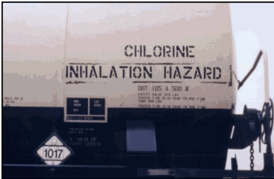
Figure F-4. Standard rail car filled with chlorine gas.
