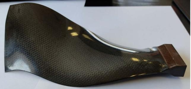
The low pressure nr. 1 disc will have 4.25 inch longer blades out of carbon fiber to pull the air into the turbine and around the turbine. The carbon fiber blades above are from a safran update. My CJ610 updated blades will have a different root and will be a little more curvature to it. I put these pictures up to give you a simulated virtual picture on the to tooling that is being designed on our CNC milling machine.
