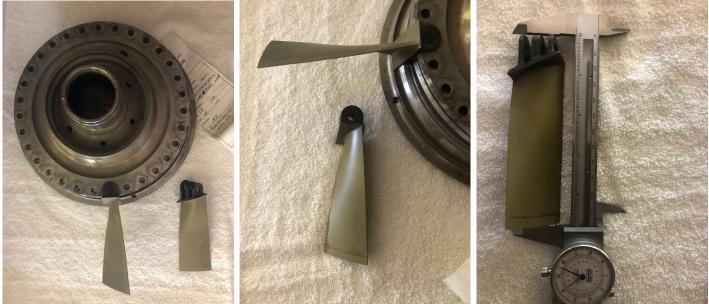
The 3 pictures above is the 1st low pressure disc with the original blades showing. The is being redesigned.
