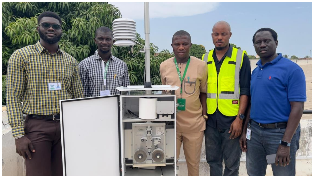
Figure 2: Installation of BAM 1022 Reference Grade Air Quality Monitor at NEA Headquarters in Kanifing, November 11th 2024
