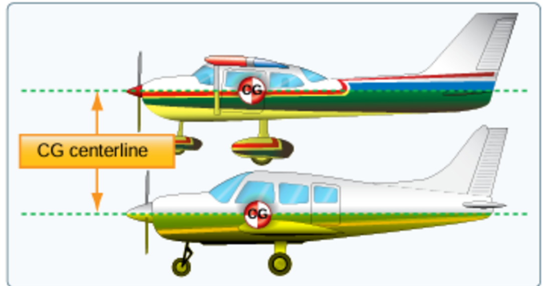
Figure 5-31. Keel area for lateral stability.
