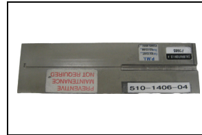
510-1406 Go/No Go Gauge, Obturator Release Rod
