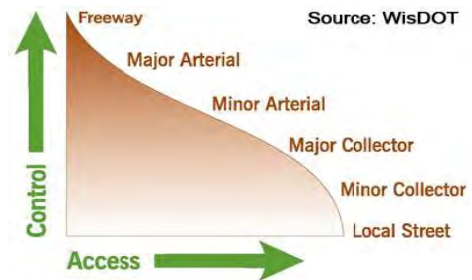
Figure 5.5: Access and Functional Classifications
