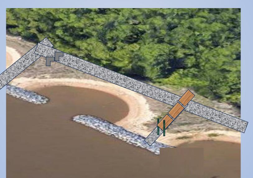
Expand the jetty system to include legs parallel to the shore.
