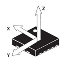
A Piezo gyroscope uses the phenomenon of Coriolis force to detect changes in angular velocity (rotation) and acceleration in three directions.
