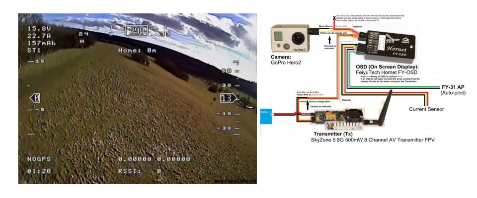
OSD can be built-in to the Flight Controller
