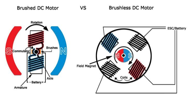
**Brushless DC motors** used in drones are 85-90% efficient whereas **brushed DC motors** are 35-40% efficient. This difference in efficiency means that brushless motors turn more power into rotational force and less is lost as friction and heat.
