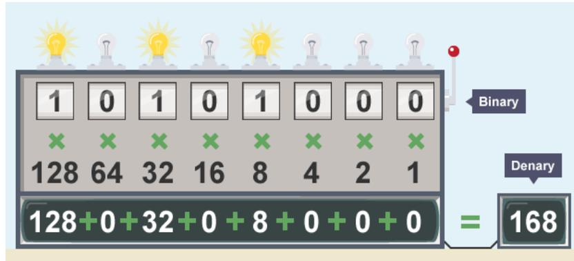
The table below shows denary numbers down the left with their equivalent binary numbers marked out below the base 2 columns. Each individual column in the table represents a different **place value** equivalent to the base 2 powers
