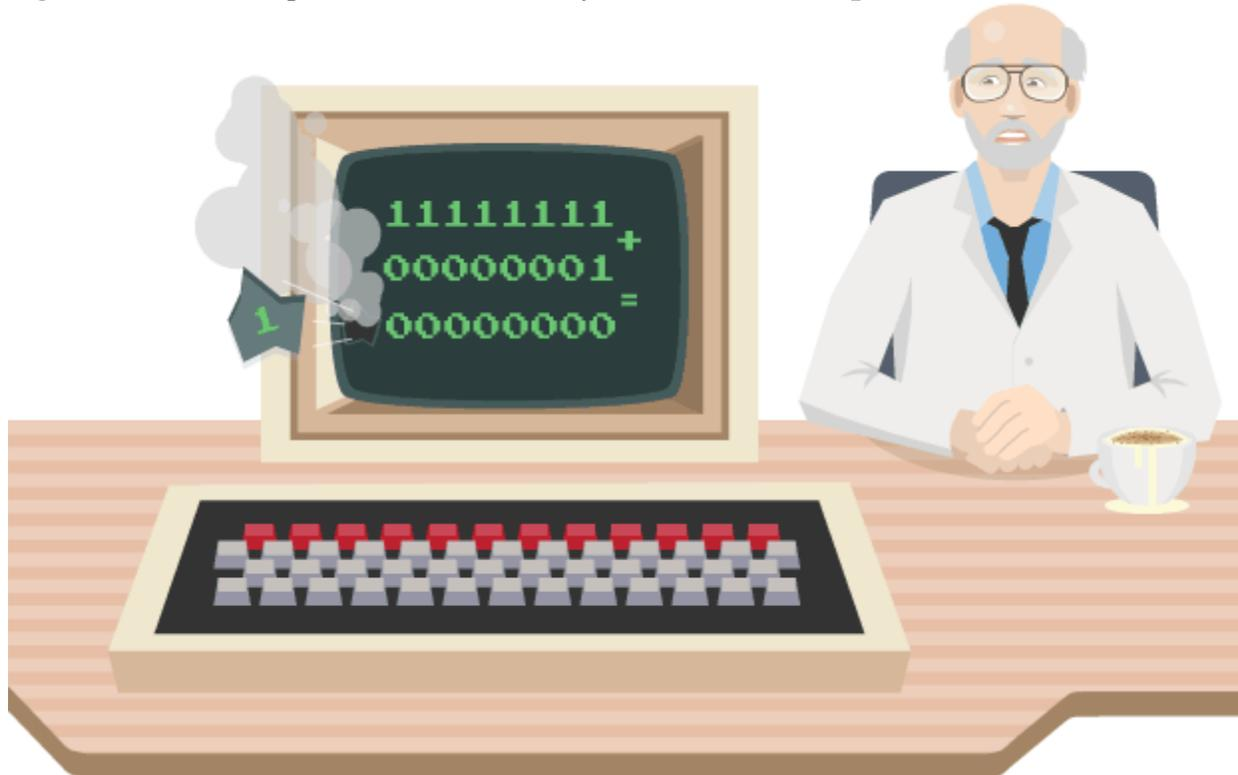
Overflow errors happen when the largest number that a **register** can hold is exceeded. The number of bits that it can handle is called the **word size**. Most CPUs use a much bigger word size than 8 bits. Many **PCs** have a 64-bit CPU. A 64-bit CPU can handle numbers larger than 18 quintillion (18,446,744,073,709,551,615 to be precise).
