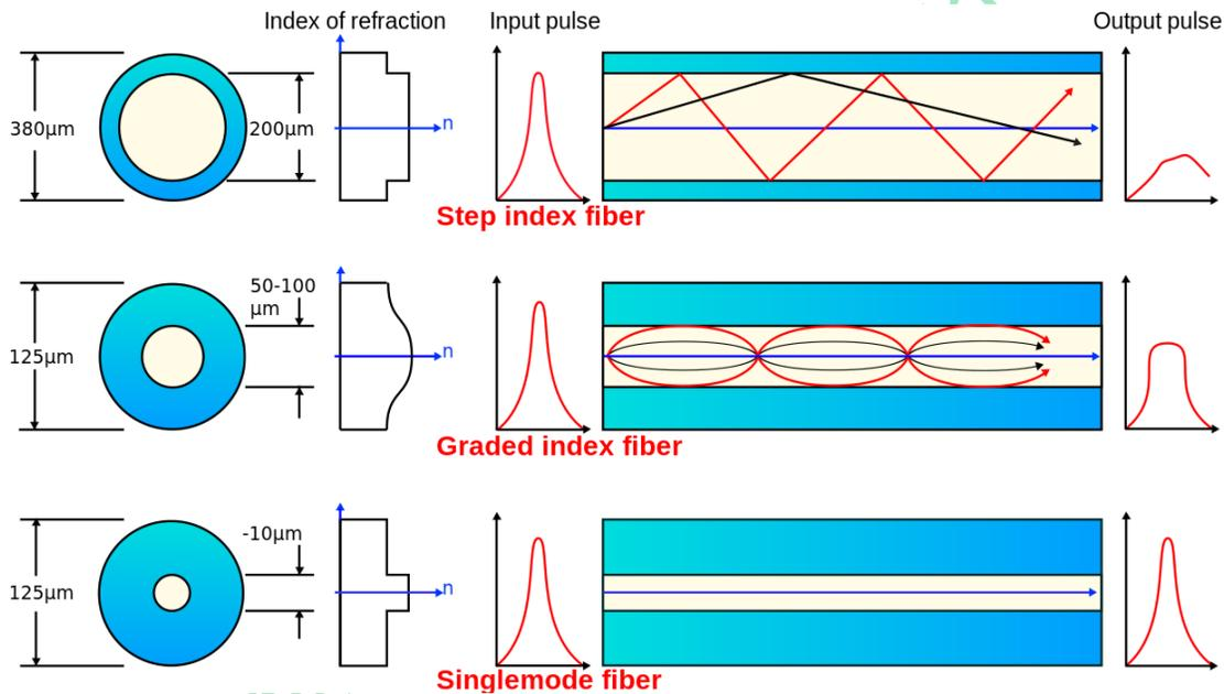
**Fiber optics** is a technology that uses glass (or plastic) threads (fibers) to transmit data. A fiber optic cable consists of a bundle of glass threads, each of which is capable of transmitting messages modulated onto light waves.
