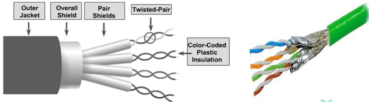
The extra covering in **shielded twisted pair** wiring protects the transmission line from electromagnetic interference leaking into or out of the **cable**. STP cabling often is used in Ethernet networks, especially fast data rate Ethernets. Contrast with UTP.
