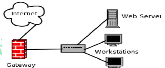
In most IP-based networks, the only traffic that doesn't go through at least one gateway is traffic flowing among nodes on the same local area network (LAN) segment -- for example, computers connected to the same switch.
