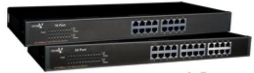
A hub is a **'dumb'** device: if it receives a message, it sends it to **every computer** on the network. This means that hub-based networks are **not very secure** - everyone can listen in to communications.
