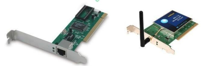
Some computers, such as laptops, have two NICs: one for **wired** connections, and one for **wireless** connections (which uses radio signals instead of wires)
