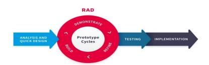
In the RAD model, the modules are developed **in parallel as prototypes** and are integrated to make the complete product for faster product delivery.
