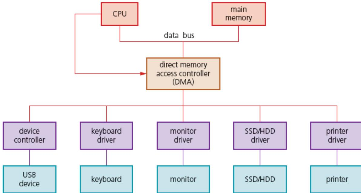
**The direct memory access (DMA)** controller is needed to allow hardware to access the main memory independently of the CPU. When the CPU is carrying out a programmed I/O operation, it is fully utilised during the entire read/write operations; the DMA frees up the CPU to allow it to carry out other tasks while the slower I/O operations are taking place.
