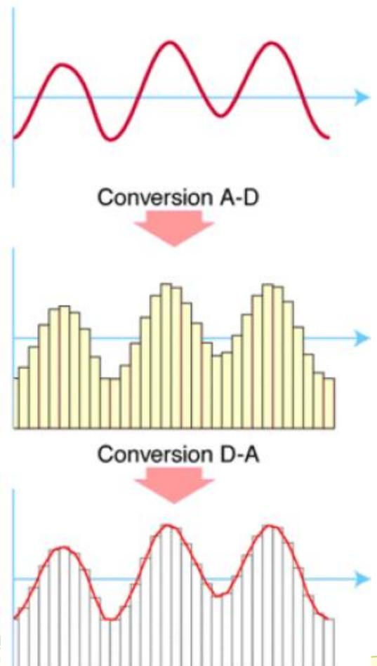
at specific intervals, called the sampling rate. Each captured wave-form snapshot is converted to a binary integer value and is then stored on magnetic tape or disk.
