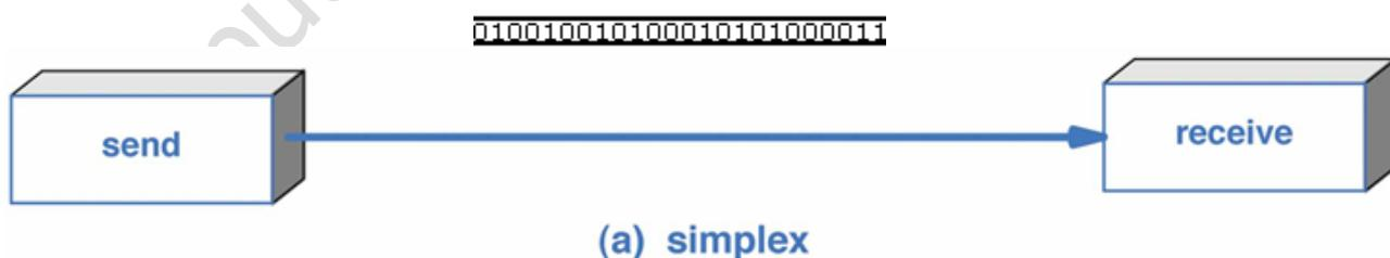
Simplex is one direction. A good example would be your keyboard to your CPU. The CPU never needs to send characters to the keyboard but the keyboard always send characters to the CPU. In many cases, Computers almost always send characters to printers, but printers usually never send characters to computers.
