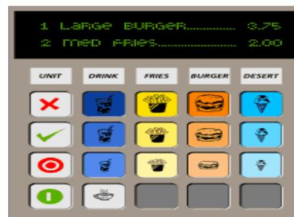
An overlay sheet with pictures or symbols is placed on the grid so that the user can tell what pressing on different areas will do. Concept keyboards are used when fast input is needed and are ideally suited to selecting from a limited range of choices such as fast food restaurants.
