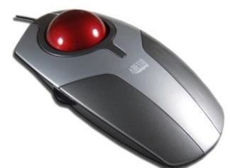
**Trackball** - similar to a mouse, this is used where extreme accuracy is needed - for example, in **CAD**, sound and video editing, and some medical imaging applications (such as **MRI** scans).
