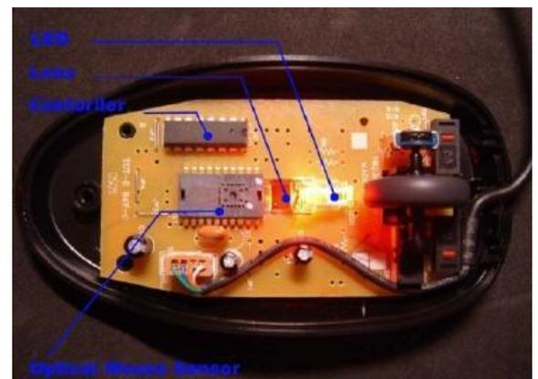
mouse and the direction of the movement of the mouse are rapidly calculated. According to the calculation, the pointer moves on the screen.
