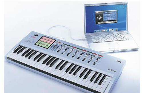
The classic MIDI synthesizer is the electronic keyboard, resembling a small piano. When you press a key on the keyboard, you hear a tone. Most new keyboards come with hundreds of different preset instrument sounds and effects from which to choose.
