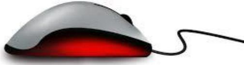
A mouse usually has two buttons, a right and left one and also a central wheel which allows you to scroll up and down the page (some mice have up to five buttons). The left and right button have different functions. Left clicking usually lets you put your cursor at a certain point on the page or lets you choose a menu item. Right clicking brings you up a list of relevant
