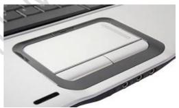
usually two buttons next to the touchpad which are used to replace the left and right mouse button.
