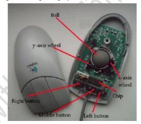
**Working Operation of mouse:** With the previous ball-rolled mice, the movement of the pointer in the computer is decided by the ball inside the mouse. So, if the ball gets damaged, or if dust gets clustered, the operation of the mouse becomes problem. When dust gathers, it takes some time to clear it too. With these disadvantages, the ball mouse was slowly moved away from the computer technology leaving the optical mouse to fill its space.
