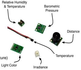
A sensor is a device that converts a real-world property (e.g. temperature) into data that a computer can process.
