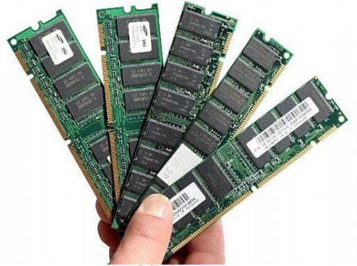
Each DYNAMIC RAM (DRAM) chip consists of a number of transistors and capacitors.
