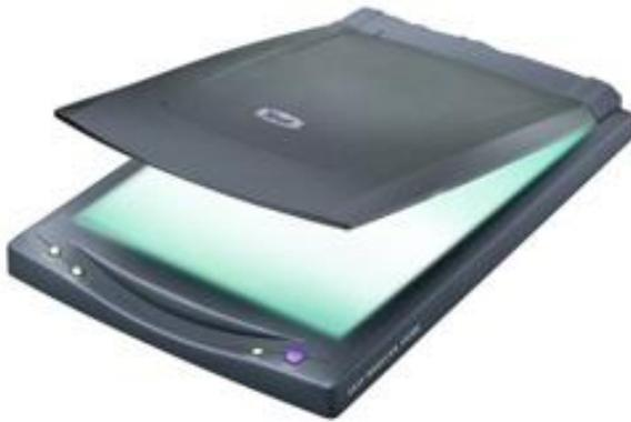
A scanner creates a digital photograph of a paper document. It scans the illuminated surface of the document with a single row of hundreds of light sensors. Each sensor produces an analogue signal that depends on the **intensity of the light it receives**.
