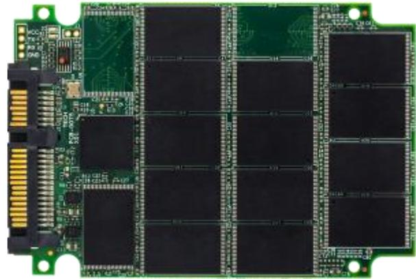
Typically SSD are made using NAND flash memory, but a DRAM based device would also be considered a solid state drive. The 2.5" form factor is most popular, but flash cards and modules such as CompactFlash, SD Card, mSATA all the way up to PCIe boards are also SSD.
