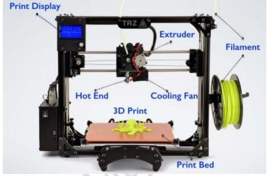
How to create a solid object using a 3D printer There are a number of steps in the process of producing an object using these 3D printers. The steps are summarised below
