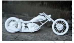
It was made from many layers (0.1 mm thick) of powdered metal using a technology known as BINDER 3D PRINTING.
