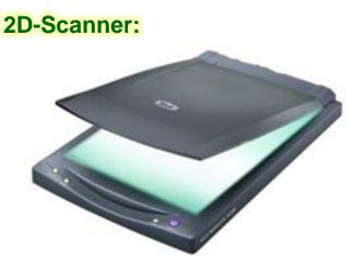
A scanner creates a digital photograph of a paper document. It scans the illuminated surface of the document with a single row of hundreds of light sensors. Each sensor produces an analogue signal that depends on the **intensity of the light it receives**.
