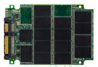
Typically SSD are made using NAND flash
