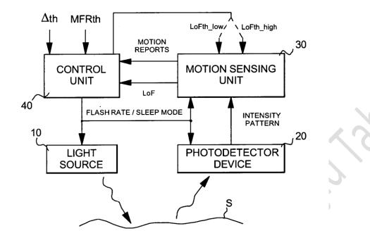
The CMOS sensor sends each image to a digital signal processor (DSP) for analysis. The DSP, operating at 18 MIPS (million instructions per second), is able to detect patterns in the images and see how those patterns have moved since the previous image.
