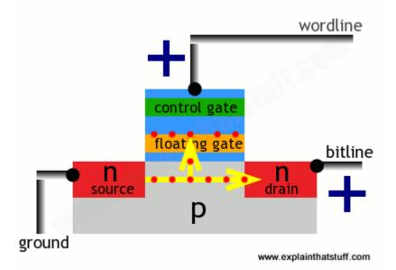
The presence of electrons on the floating gate is how a flash transistor stores a one. The electrons will stay there indefinitely, even when the positive voltages are removed and whether there is power supplied to the circuit or not. The electrons can be flushed out by putting a negative voltage on the wordline—which repels the electrons back the way they came, clearing the floating gate and making the transistor store a zero again.
