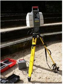
Data is collected in relation to an internal coordinate system and therefore to collect data where the scanner is in motion the position of the scanner must be determined.
