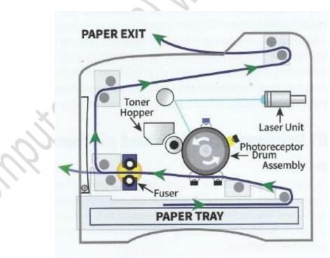
Figure 3.06 A schematic diagram of a laser printer
