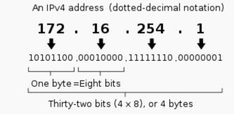
Decomposition of an IPv4 address from decimal value to its binary value.
