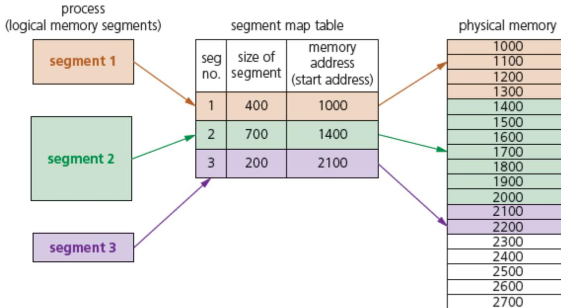
The segment map table in **Figure** contains the segment number, segment size and the start address in physical memory.
