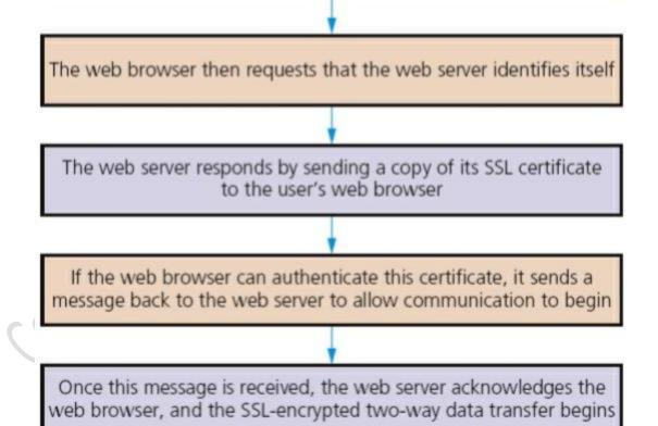
**TRANSPORT LAYER SECURITY (TLS)** is similar to SSL but is a more recent security system. TLS is a slightly modified version of SSL
