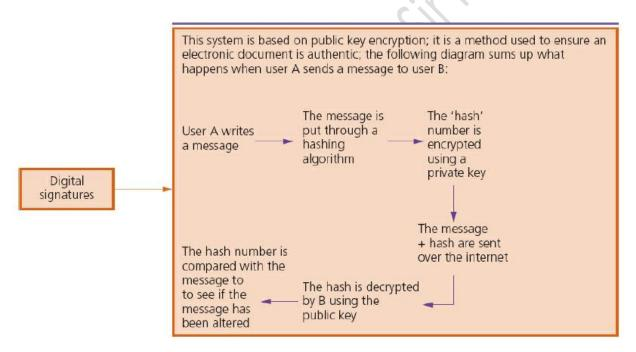
There is a disadvantage in using this method of applying a digital signature in that it is associated with an encryption of the whole of a message.
