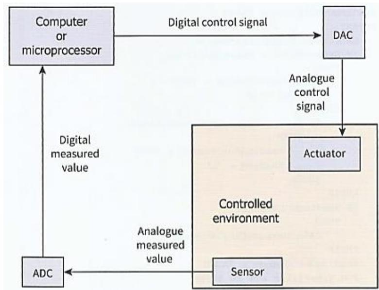
The system shown in Figure involves a continuous process where measurement is made and then, if needed, a control action is initiated. Following this control action, a measurement is taken again. There is therefore an element of feedback in the system.
