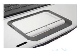
usually two buttons next to the touchpad which are used to replace the left and right mouse button.
