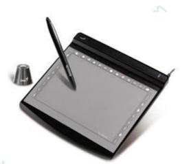
A graphics tablet consists of a flat pad (the tablet) on which you 'draw' with a special pen. As you draw on the pad an image is created on the computer monitor from within the application that the tablet is connected to.
