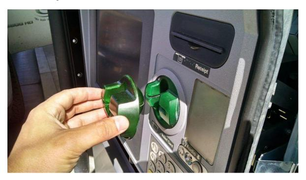
Credit card skimmers are often placed over the card swipe mechanism on ATMs and gas stations,
