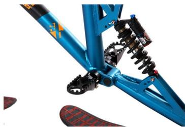
The lower gravity center and bigger platforms foot rests are providing much more balance and control to ride down with skid turns. With these improvements the Skibike offers a lot more possibilities to ride.
